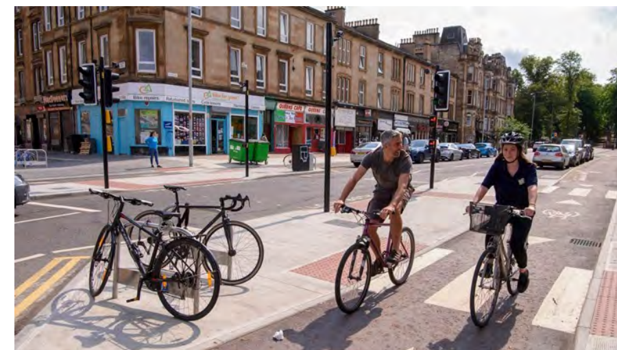
Protected cycle track, catering for side-by-side cycling
